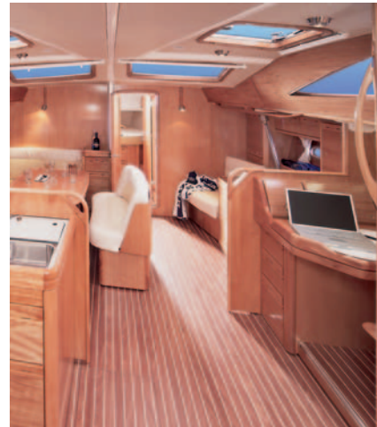
Open interior layout with eight fixed hull ports, two deck skylights, nine opening hatches with roller shades and two non-opening panoramic windows for enhanced light and cross-ventilation
