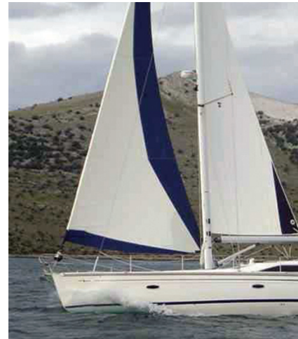
Double spreader Selden mast, conventional, furling or fully-battened mainsail, adjustable pneumatic boom vang and adjustable backstay
